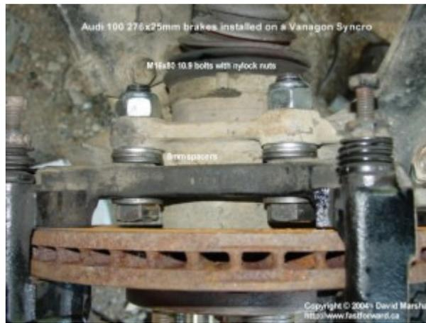
**Audi Caliper Carrier mounted on a Vanagon Syncro Hub**
